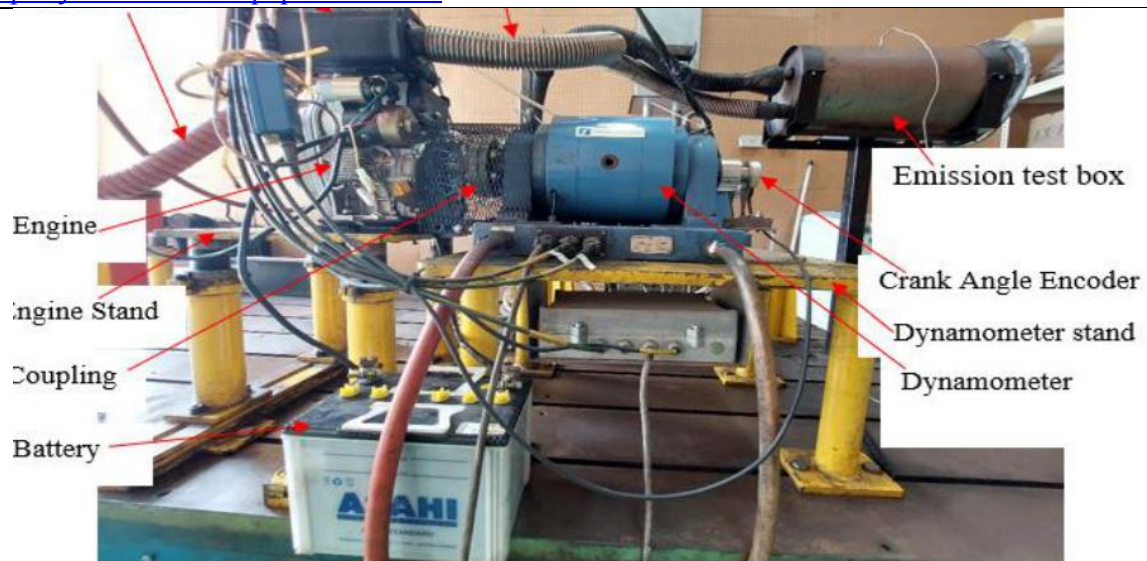
Figure 5. Engine-dynamometer-emissions test rig used for single-cylinder evaluation of hybrid magnetite/alcohol additives in palm biodiesel operation [15].
